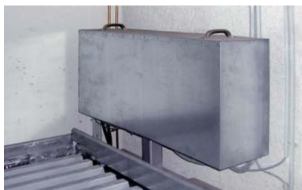
Sound insulation hood for the power unit
