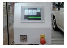
Operation by touch screen with key switch and emergency-stop. With brief operating instructions fastened on the wall and cabling to the power unit.
